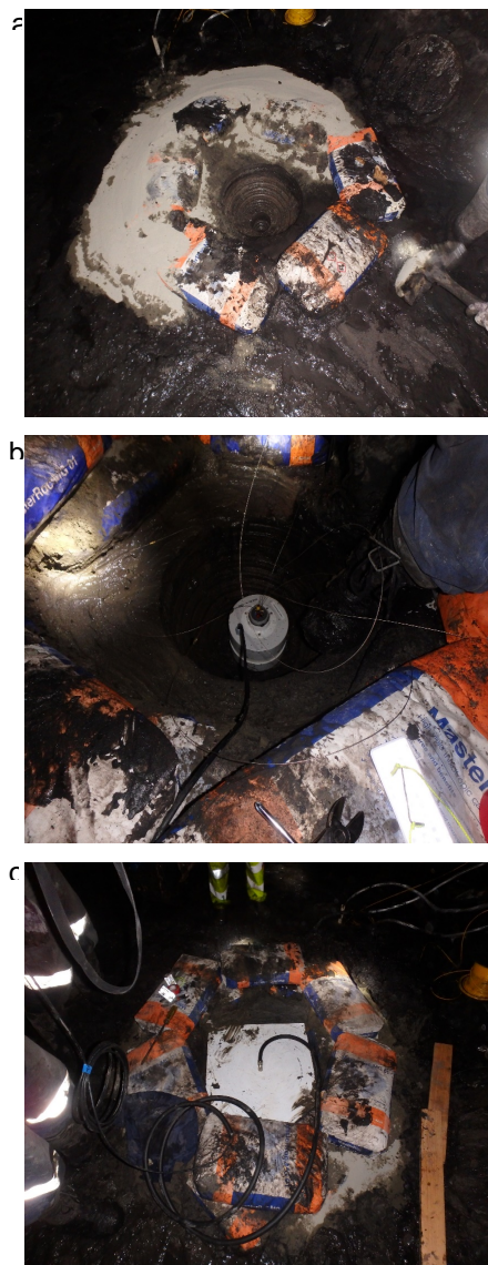
Figure 12: Shear strip and remote reading tell-tale installed in Mine A
