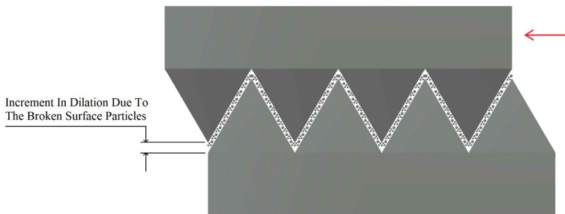
Figure 9: Increment in dilation of unfilled joint due to damaged surface particles, designed in AutoCAD
