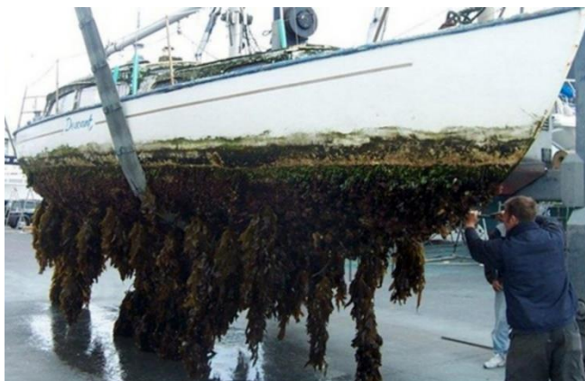
650 Figure 11: Fouling costs upon the attachment to ship hull which cause serious problems in shipping industry. Reproduced with permission from Editec Group.
