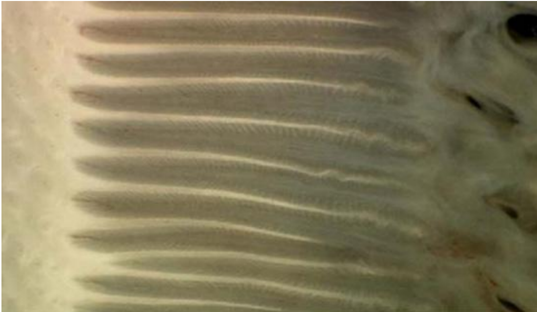
Figure 1 - Interface between high toughness (left) and low toughness (right) epidermal layers of horse hoof showing interdigitated transition region, image courtesy of Dr Chris Pollitt, University of Queensland.
