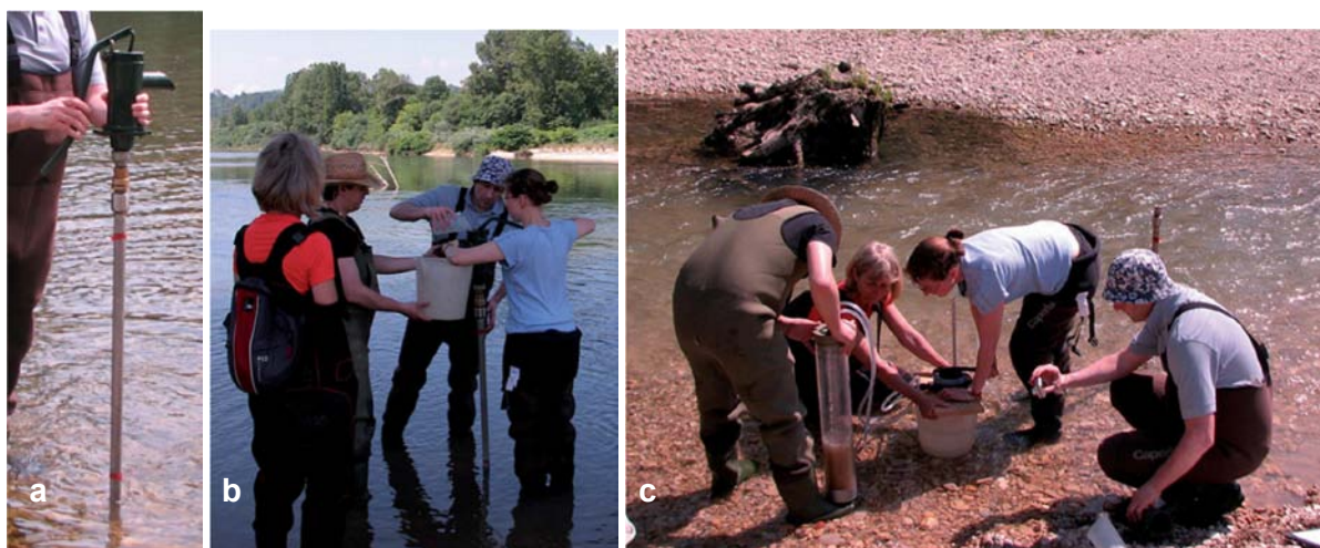
Figure 4.12 Equipment and mode of operation for two methods used to pump invertebrates from subsurface sediments: (a) the Bou-Rouch pump and (b) its operation; (c) vacuum-pump sample collection. Further information is provided in Stubbington et al. (2016).
