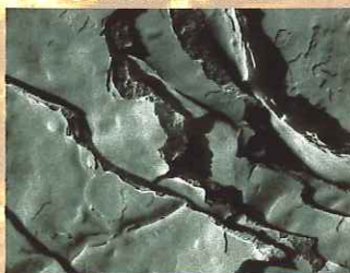
FFEM micrograph corresponding to two PC vesicles showing diameters of about 180 nm, in agreement with the DLB results
