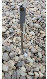
2 insertion devices in each point of the mesh for pressure sensors.
