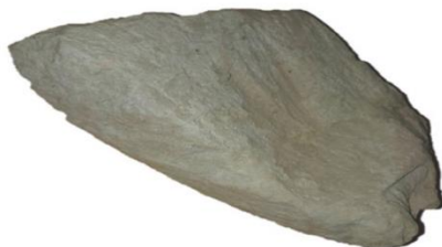
Figure 1: Natural (crude) clayey diatomite from Bitola region.
