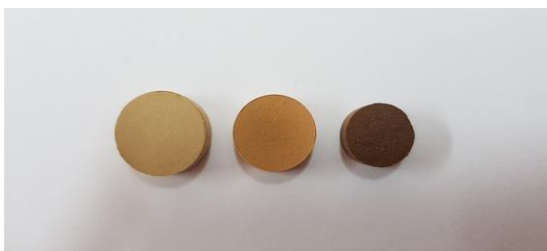
Figure 8: Shrinkage and the obvious change in color of cylinders of clayey diatomite sintered at 800, 1000 and 1200°C for a period of 60 min.
