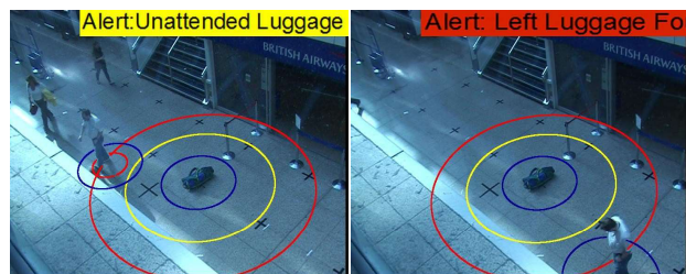
Figure 11: A sample from S08. First the person leaves the 3m radius. After 25s an alert will be set
