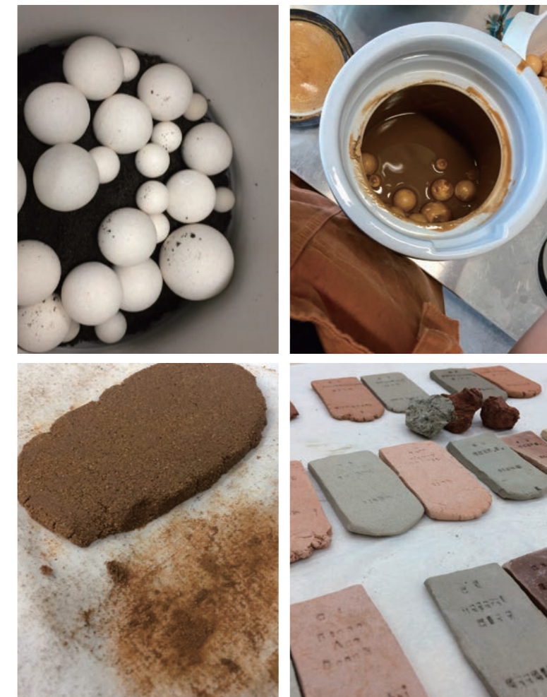
Figure 12. (top) Processing the gathered soils by using the ball mill machine. (bottom) Making test pieces with the gathered soils.
