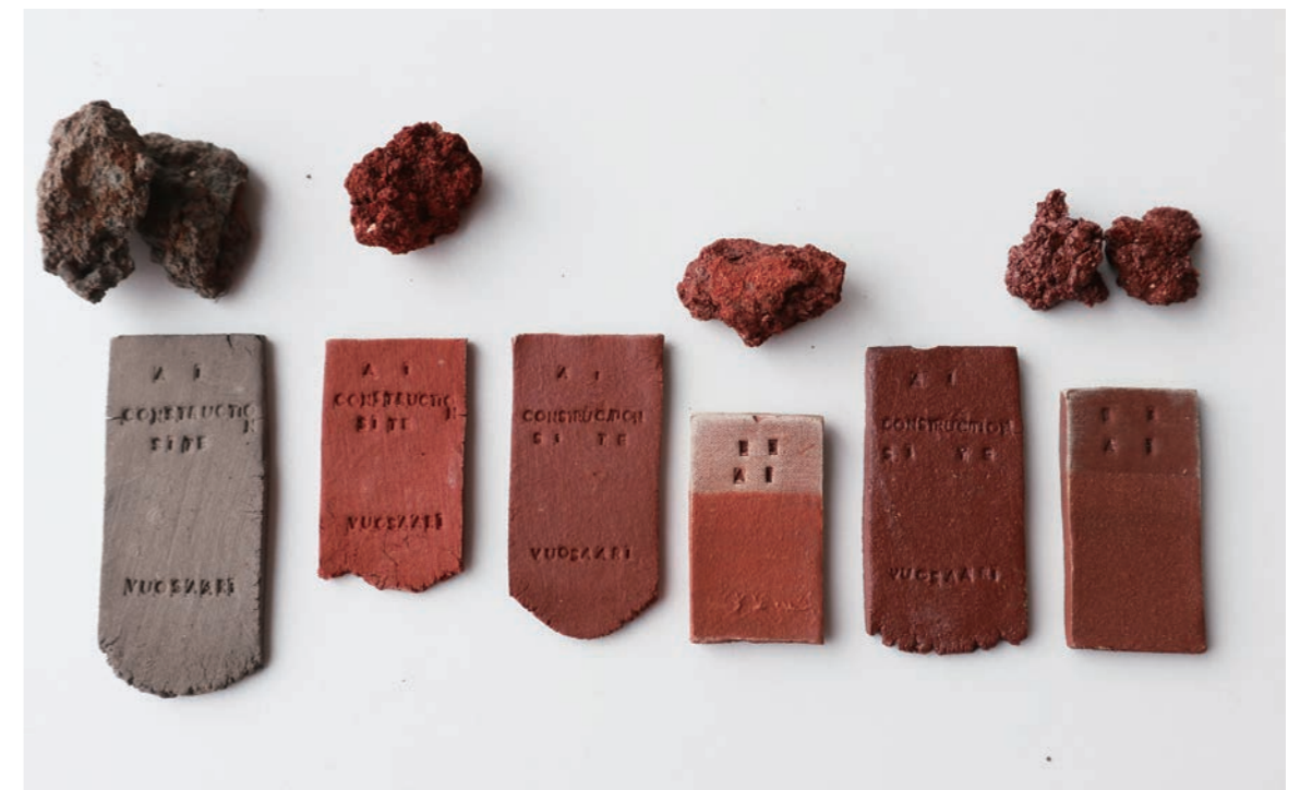
Figure 14. Selections of the test pieces. (top) Natural clay soil and fired samples from Sipoo, (bottom) Soil and fired ceramic samples from the Vuosaari construction site.
