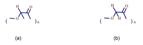
Figure 1.5. Chemical structure of (a) poly(lactic acid) and (b) poly(glycolic acid) (adapted from Hincal and Calis, 2000).
