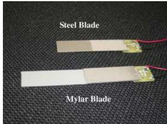
Figure 2.3. Two piezoelectric fans (mylar and steel blades) tested to characterize the influence of operating parameters (Kimber et al., 2009b).
