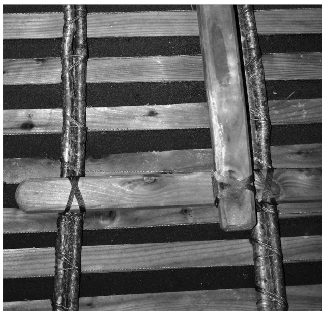
Ill. 3 & 4: The ribs of this currach (North Donegal, 1999; NMIF 1999:351) are of rough hazel and are tied to the long laths with cords – a most ancient technique.
