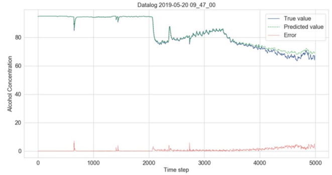
Fig. 10. Kalman filter output on 70% reflux ratio
