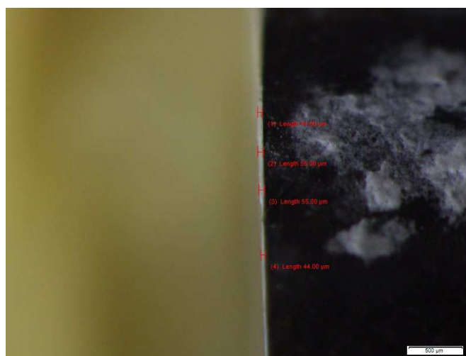
Fig. 3 Scanning electron microscope of hydroxyapatite-coated thickness at 5V for 5 minutes deposition
