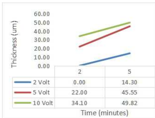
Fig. 4 Thickness curve of hydroxyapatite-coated titanium
