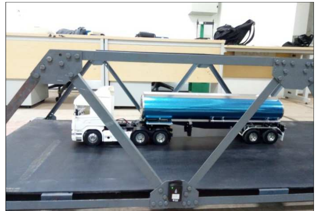
Fig. 2 Miniature truck to simulate the traffic load
