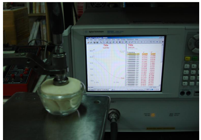
Fig. 3. Agilent N5230A VNA with HP 85070B dielectric probe.
