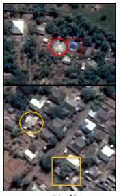
(a) Before (b) After Fig. 10 Building loss detected after Lombok earthquake from Pleiades imagery acquired on a) 1 May 2018 and b) 7 August 2018
