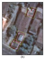
Fig. 7 Delineation accuracy for building from the reference map in white and red as tolerance accuracy for 0.5m from reference (for level 2 map scale standard), yellow as tolerance accuracy for 2m from the reference map (for level 3 map scale standard), while image b) shows the building delineation for area less than 45  $m^2$
