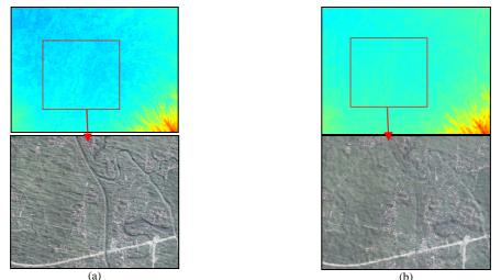
(a) (b) Fig. 4 Comparison of a) TSX DSM (9m) and b) ALOS PALSAR DSM (12.5 m)
