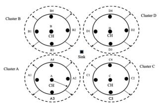
Fig. 2 Layering wireless sensor network cluster
