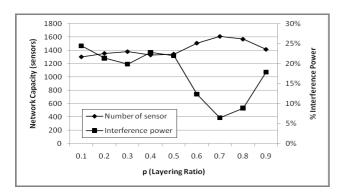
Fig. 3 Effect of layer ratio on network capacity and interference
