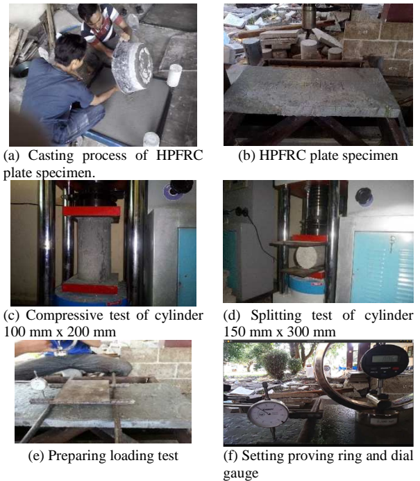
Fig. 4 Preparing and testing HPFRC cylinder and plates
