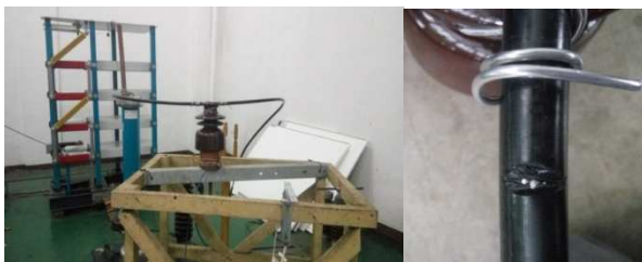
Fig. 4 Voltage impulse testing
