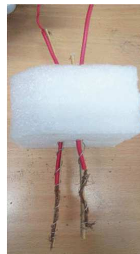
Fig. 3. Homemade Soil Moisture Sensor [39]
