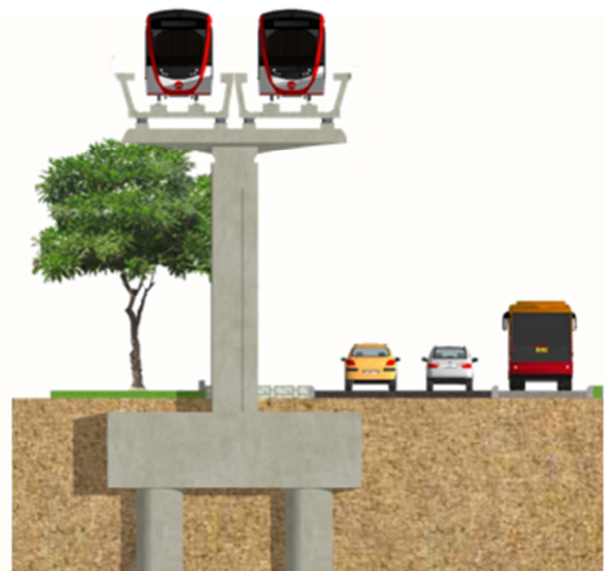
Fig. 3 Typical structure of LRT Jabodebek
