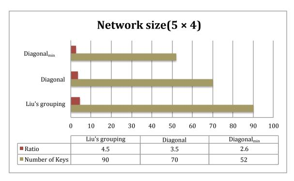
Figure 5.18: Total number of keys and key-to-sensor ratio for a  $5 \times 4$  network.
