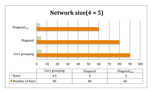
Figure 5.10: Total number of keys and key-to-sensor ratio for a  $4 \times 5$  network.
