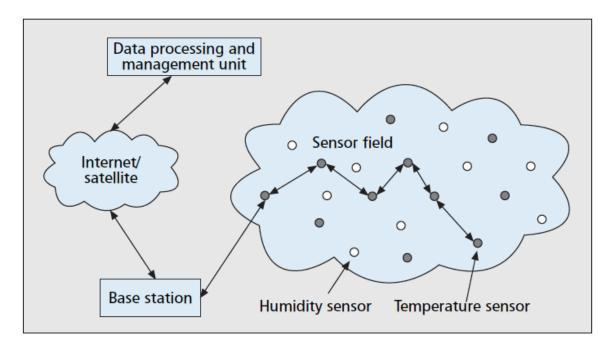
Figure 2.1: Simplified architecture of a wireless sensor network [19].
