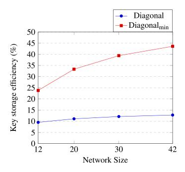
Figure 5.15: Increase in key storage efficiency where n < m.
