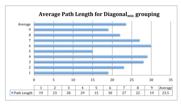
Figure 5.34: Average pathkey length using diagonal<sub>min</sub> grouping for a  $3 \times 3$  network, where n = m.
