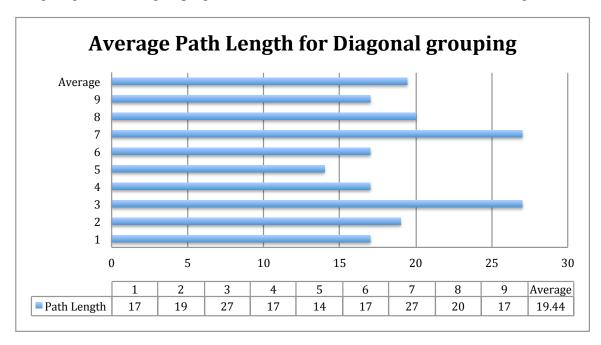
Figure 5.32: Average pathkey length using diagonal-based grouping for a  $3 \times 3$  network, where n = m.
