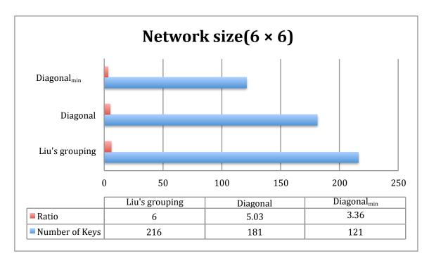
Figure 5.4: Total number of keys and key-to-sensor ratio for a  $6 \times 6$  network.
