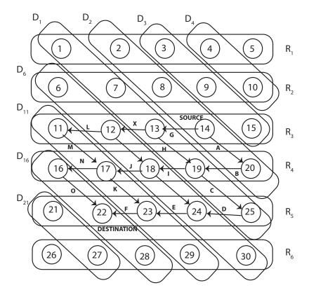
Figure 4.14: Pathkey establishment for diagonal-based grouping for  $6 \times 5$  network.
