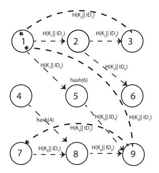
Figure 4.7: Distribution of hash keys in diagonal<sub>min</sub> grouping for a  $3 \times 3$  network
