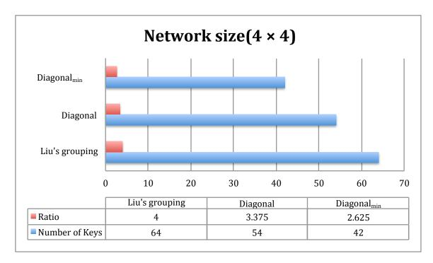
Figure 5.2: Total number of keys and key-to-sensor ratio for a  $4 \times 4$  network.
