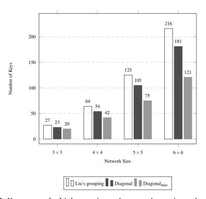
Figure 5.5: Key storage for Liu's grouping and proposed groupings where n = m.
