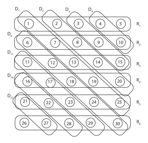
Figure 5.46: A  $6 \times 5$  network, where n > m using diagonal-based grouping.
