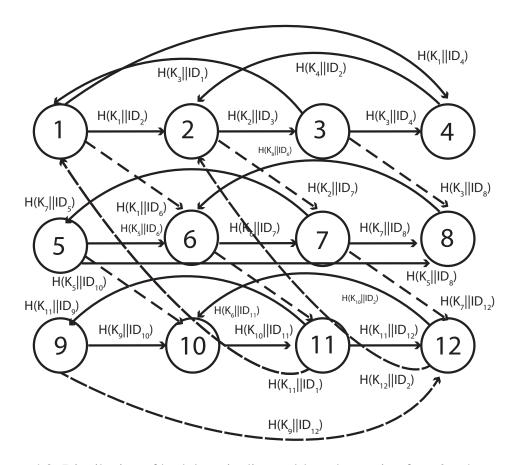
Figure 4.8: Distribution of hash keys in diagonal-based grouping for a  $3 \times 4$  network.
