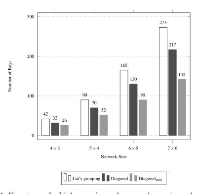
Figure 5.21: Key storage for Liu's grouping and proposed groupings where n > m.
