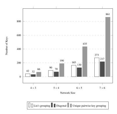
Figure 5.22: Key storage for unique pairwise key grouping and proposed groupings where n > m.
