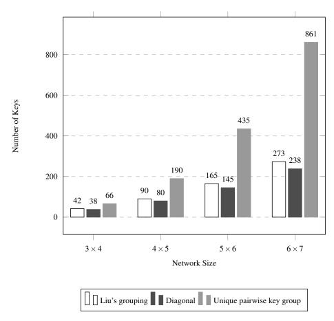
Figure 5.14: Key storage for unique pairwise key grouping and proposed groupings where n < m.
