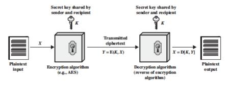
Figure 2.2: A simplified model of conventional encryption [2].
