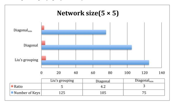
Figure 5.3: Total number of keys and key-to-sensor ratio for a  $5 \times 5$  network.
