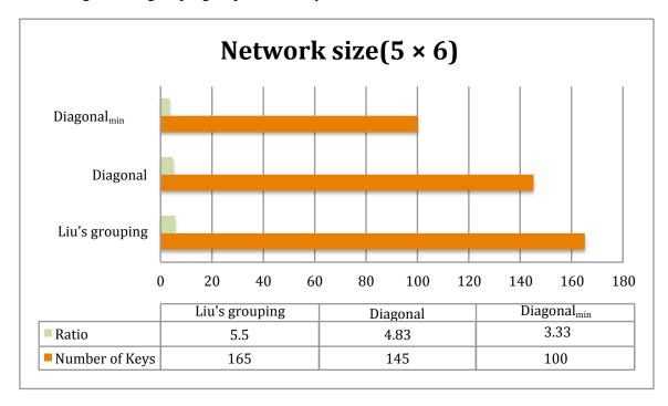
Figure 5.11: Total number of keys and key-to-sensor ratio for a  $5 \times 6$  network.
