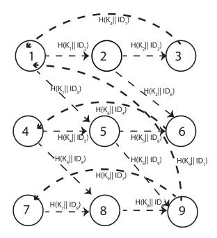
Figure 4.6: Distribution of hash keys in diagonal-based grouping for a  $3 \times 3$  network
