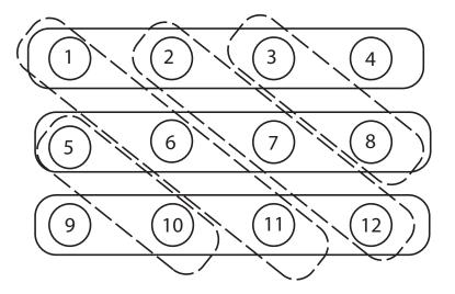
Figure 5.38: A  $3 \times 4$  network, where n < m using diagonal-based grouping
