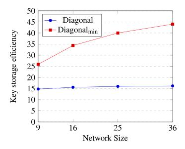
Figure 5.7: Increase in key storage efficiency where n = m.
