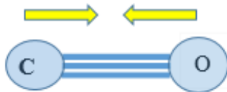
Figure 2.7: Stretching mode of CO.
