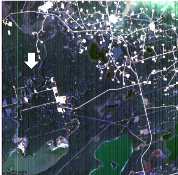
Figure 3.7: CHRIS radiance RGB (bands 24, 7 and 12) imagery captured in mode 1 over Cold Lake, Alberta. Major striping is noted by the white arrow.
