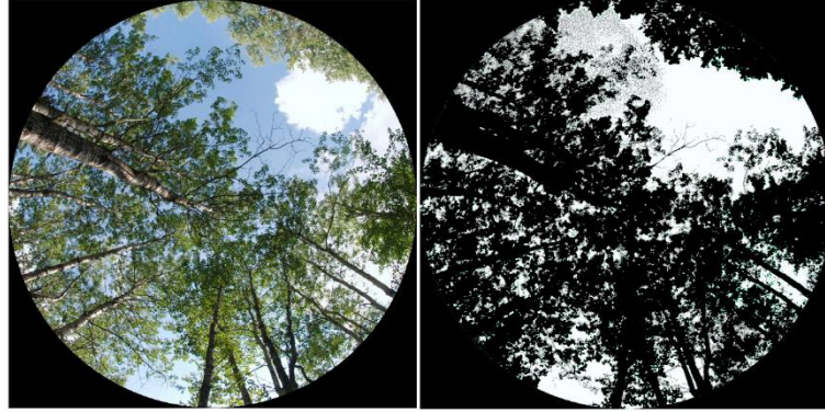
Figure 3.5: Hemispherical photograph (left) and classified image using the CAN-EYE software (right); black corresponds to tree, white to sky or soil (depending on the orientation of the image), and grey is mixed.
