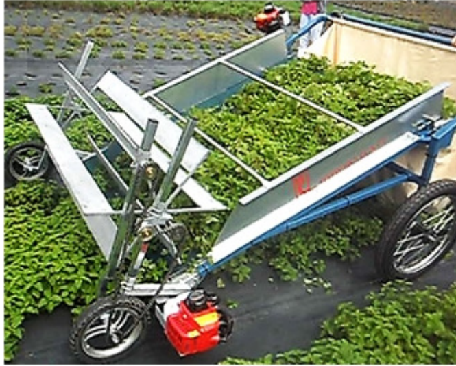
Figure 5: MAP harvesting machine by McLeça
