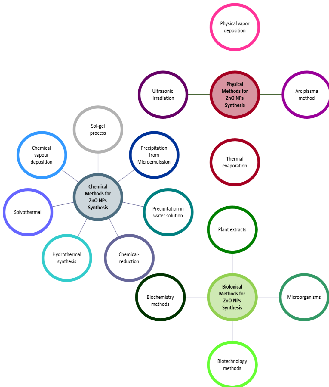
Figure 2: The variety of physical, chemical and biological methods to synthesize ZnO nanoparticles. (Reproduced from: Kolodziejczak-Radzimska and Jesionowski, 2014; Król et al., 2017 )
