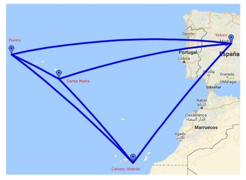
**Figure 1.** The RAEGE network, covering most of Macaronesia, or the central and north-west Atlantic Ocean. When fully deployed, RAEGE will have VLBI stations spread over the American, European and African plates.
