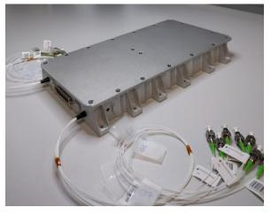
Figure 3. Fully assembled multi-core array fiber amplifier
