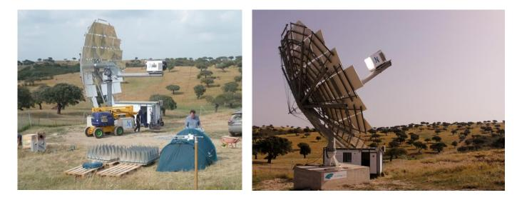
**Figure 11**. Biostirling project (FP7) in action in Herdade da Contenda, Moura. Two world first times: first time in the world a solar concentrator with a hybrid Stirling engine in its focus was trialled; first time a radioastronomical system was fed with solar power. Left: solar concentrator and modules of SKA Mid Frequency Aperture Array. Right: Dish-Stirling concentrator unit in routine Sun operation; we can see the bright focus spot, at ~700°C.
