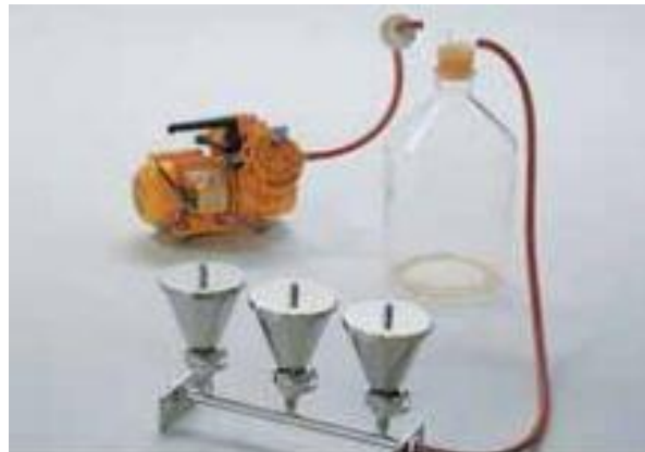
Figure 3 - Three branched manifold membrane filter system used for waters and wines. Image adapted from Just & Regnery (2008).
