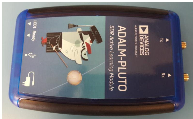
Figura 2.4: ADALM-PLUTO, da Analog Devices.
