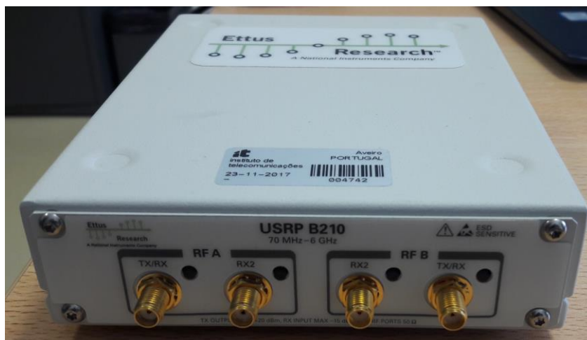
Figura 2.6: USRP B210, da Ettus Research/National Instruments.
