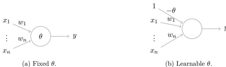
Figure 2.3: Perceptrons. In one (left) the threshold is fixed, whereas in the other (right) it is learnable.
