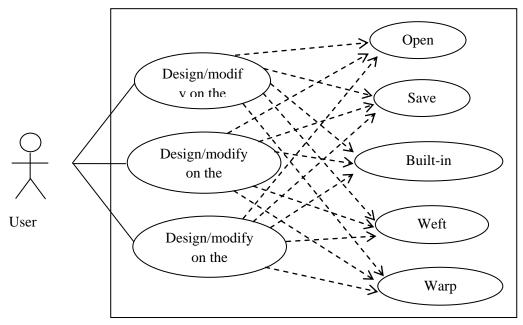
**Figure 4.6** A *Use Case* diagram of the LT-Weave module
