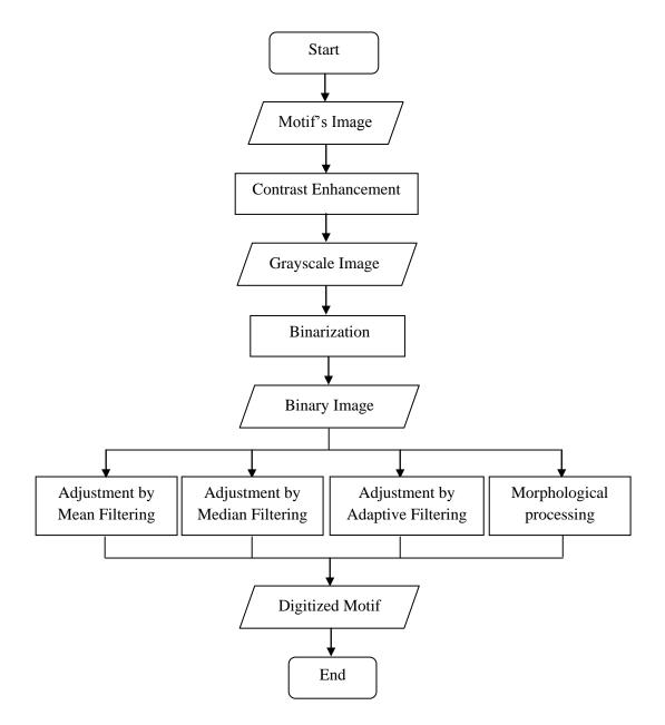
**Figure 3.15** A flowchart for extracting and digitizing motif by image processing techniques
