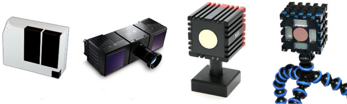
Figure 1.3: Shown are different models of time-of-flight cameras. (a) Argos 3D-P100 with up to 160 fps and 160 \times 120 pixels [6], (b) PMDs CamCube with 204 \times 204 pixels and SBI [67], (c) SwissRanger 4000 of MESA Imaging having 176 \times 144 pixels [81] and (d) TOF-camera having 176 \times 144 pixels
