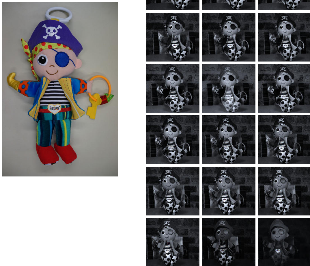
Figure E.4: The pirate scene. The RGB image is taken with a Sony ILCE-7E camera. It is not representing the ground truth color but illustrates the color distribution of the object. The heterogeneous light field is captured with a PCO edge 5.5 camera. The captured heterogeneous light field contains 21 images (top left to bottom right). The filters employed have a full width half mean value of 10 nm with the given mean values: 400 nm, 450 nm, 500 nm, 515 nm, 532 nm, 550 nm, 560 nm, 589 nm, 600 nm, 650 nm, 700 nm and back down to 400 nm.
