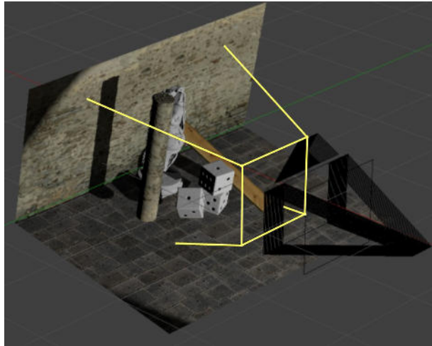
Figure D.6: Shows a loaded setup defined with the light-field camera configurator. Now aside the camera array also the related frustum is displayed. Scenes can now be positioned inside the frustum.
