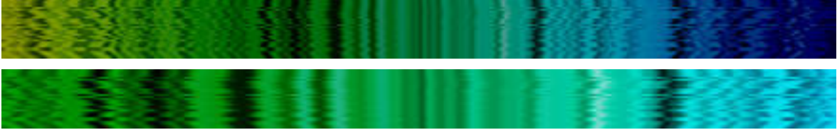
Figure 3.7: Inaccuracy in camera focal length causes jitter with a parabolic distribution in EPI space. The top image shows the jitter distribution of a plane located at a distant position of the camera array, and the bottom shows the same plane close to the camera. Jitter distribution looks like a zoomed part of the top image which means that the jitter ratio increases.
