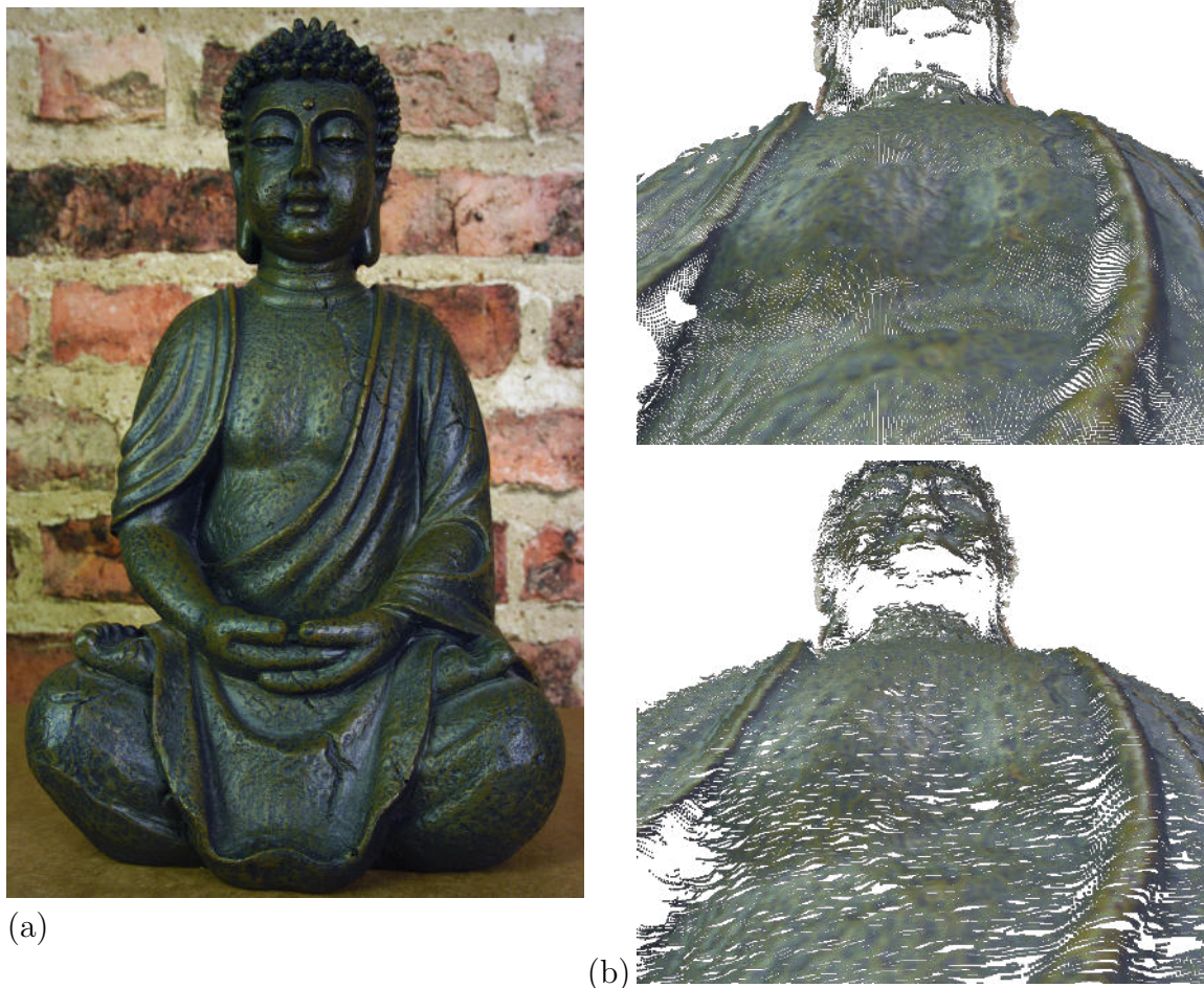
Figure 2.5: (a) shows the center view image of the processed light field which consists of 21 images. (b) shows the point clouds of the 2.5D Structure Tensor on the top in contrast to the 2D Structure Tensor at the bottom. It illustrates that the 2.5D Structure Tensor interconnects the EPI rows (horizontal direction), while the 2D Structure Tensor keeps them independent. Thus much smoother surfaces are possible.
