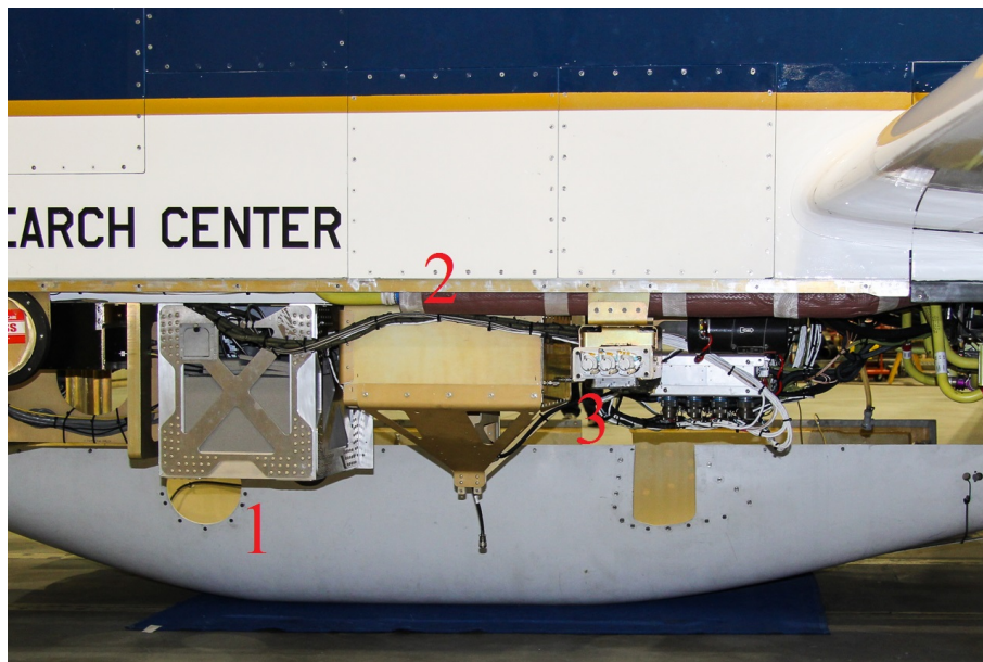
Figure 5.2: Photo of the instrument integrated in zone 25 (location see 4.2), the unpressurised belly pod of the GH, without fairing. 1) spectrometers assembly 2) fiber bundles 3) telescopes.
