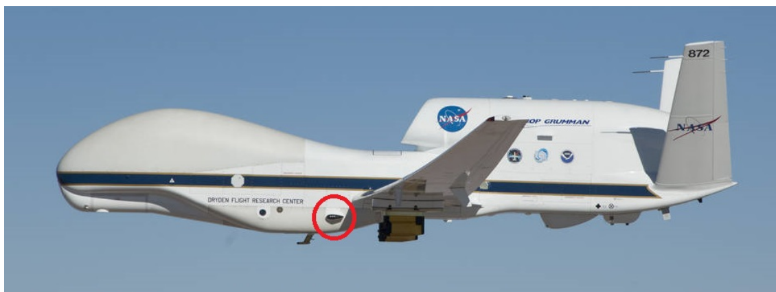
Figure 4.1: The Global Hawk aircraft during flight. The telescopes of the mini-DOAS instrument are marked with a red circle. Credits: NASA Photo / Tom Miller
