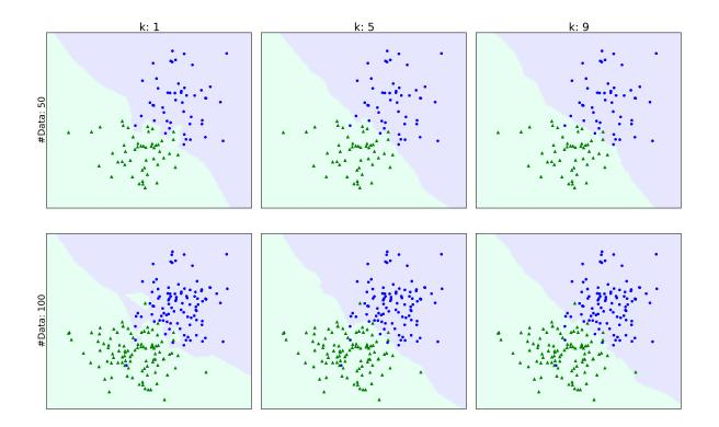
Figure 2.8: Classification depending on different choices of k in a nearest neighbors classifier. The background color encoding highlights the course of the classification boundary, which is very abrupt (smooth) for low (high) values of k.
