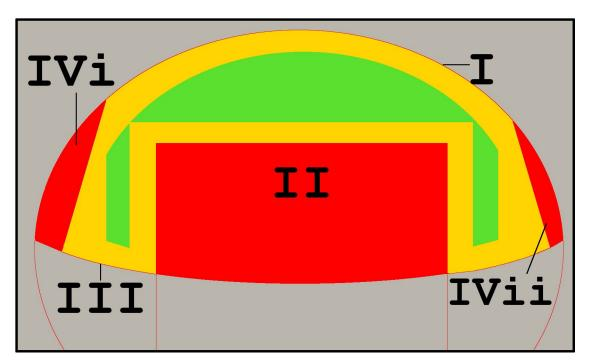
**Figure C.2:** The different regions of the patrol field. The forbidden/flagged regions are marked red/orange, the preferred region is marked green.
