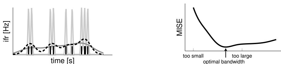
Figure 1.6: Error criterion for the bandwidth parameter and the optimal bandwidth. Left: True underlying rate (black dashed line), noisy firing rate estimate with a too narrow bandwidth choice (light gray), oversmoothed firing rate estimate with a too large bandwidth (dark gray). Right: mean integrated squared error (MISE) quantifies deviation from the underlying rate (on the left) as a function of the bandwidth, MISE values for the two non-optimal firing rate estimates shown in the left plot are indicated as marks on the x-axis.
