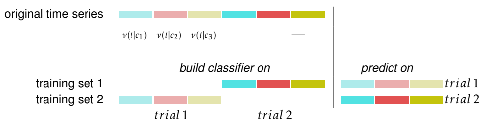
Figure 2.5: Simplified illustration of the m-fold cross-validation scheme with l=2 trials, k=3 response-classes, class labels are color-coded
