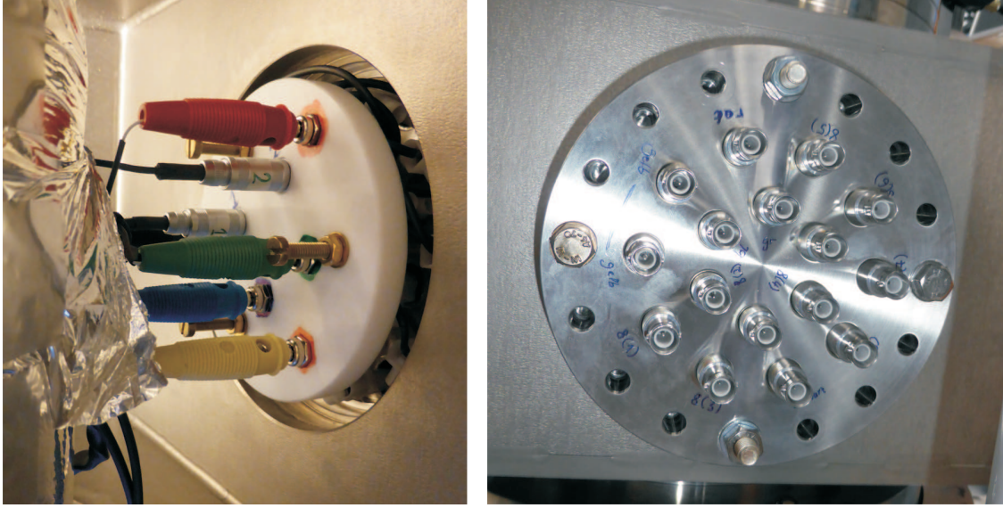
Figure 4.23: Photographs of the HV feedthroughs, with Lemo and banana sockets at a Teflon flange on the vacuum side (left) and SHV connectors on the atmospheric side (right).
