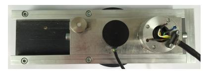
FIGURE B.4: Picture of the LED setup which provides switching between two LED lamps (without any daylight irradiation during the change of the LED lamp). It is designed to be mounted on a UV window of a UHV chamber for UV/vis irradiation experiments.
