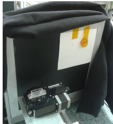
(b) Fully closed outer plate with a ^{22}\text{Na} source.
