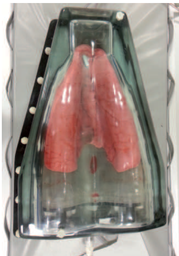
Figure 3.3: Ex-vivo porcine phantom. Thorax phantom containing an excised porcine lung attached to a vacuum pump. Image courtesy of Jascha Zapp.
