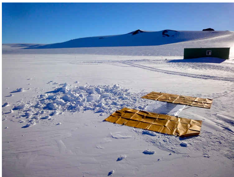
Figure 6.23.: Part of the snow pit experiment: The instrument was placed inside a hole dug into the snow on the ice shelf and covered with PTFE foil to inhibit the exchange of air but still allow sunlight to enter the chamber.
