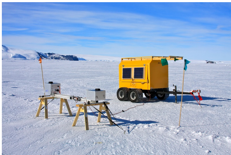
Figure 6.19.: The CE-DOAS instrument at Cape Evans. Power was supplied by six lead acid batteries located inside the yellow trailer and the two solar panels visible on its side.
