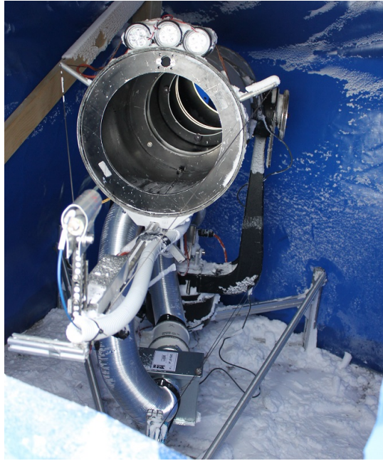
Figure 4.9.: The telescope of the LP-DOAS system. Photo courtesy of Denis Pöhler.
