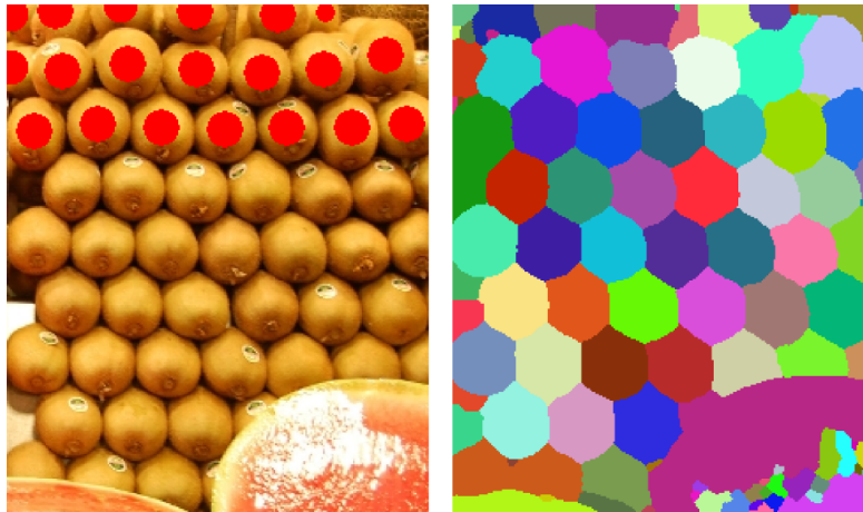
Figure 4.1: Segmentation example. Each connected component of the user scribbles is treated as an individual label and the decision tree is trained using must-link constraints inside each component and cannot-link constraints between label components. The resulting tree learns an edge model consistent with the user-provided constraints and successfully generalizes to the unlabeled part of the image, where it segments many objects successfully.
