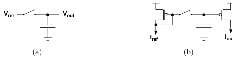
Figure 6.1: Simplified schematic showing the basic concept of capacitive storage cells. (a) shows a cell storing voltages, (b) a corresponding design for currents.
