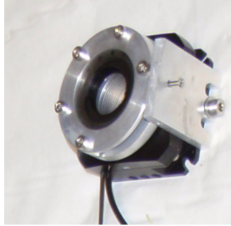
Figure 3.5: Photographic picture of the motorized zero-aperture iris used in the setup presented in this work. With the iris mounted on the 0.035 mrad step size motor the beam diameter of the divergent VIS pulse can be controlled with high precision.
