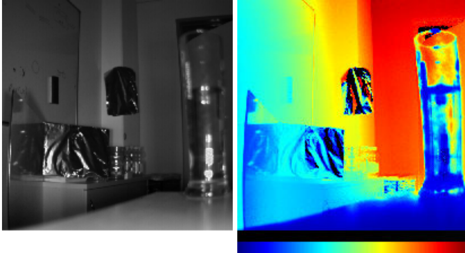
Figure 5.6: Left: intensity image of real example scene with problematic content. Right: Depth map of same scene. Depth estimations on reflecting (aluminum foil) or transparent (water glass) surfaces differ wildly.
