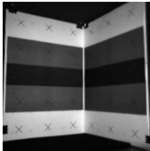
Figure 5.28: Intensity image of RealCorner . The black crosses where used as features for the 2D-to-3D pose estimation.
