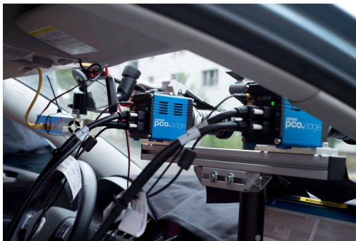
Figure 3.10: Cameras mounted in test vehicle. The stereo baseline was at 30 cm
