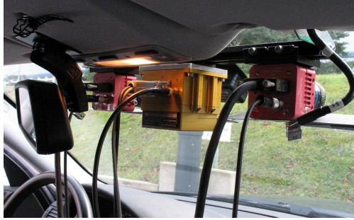
Figure 3.3: Stereo rig mounted in car. The GPS/IMU unit is located in the center.
