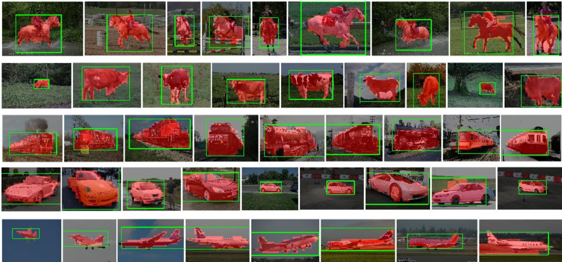
Figure 4.7: Detection examples for certain PASCAL VOC 2007 categories. The cells corresponding to the object foreground are grouped and used for detection.
