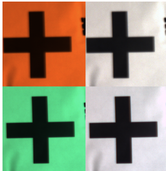
Figure 3.11: Two images captured under strong red light (top left) and white light (bottom left) illumination. The images with white color correction are shown here (right).
