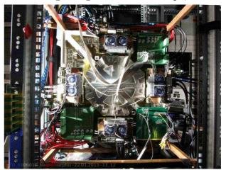
Figure 1: Wafer Scale Integrated (WSI) System. The Wafer is situated under the silver-coloured bracket in the centre - taken from BrainScaleS homepage [34].
