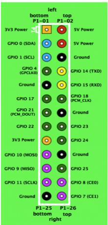
Figure 7: GPIO pin numbering on the Raspberry Pi P1 header [21].
