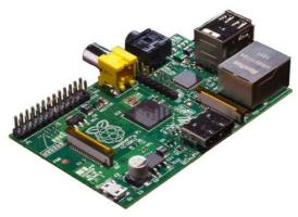
Figure 3: Raspberry Pi – size as big as a credit card. The header P1 is the one at the very left, equipped with pins. This header is used with the ribbon cable.
