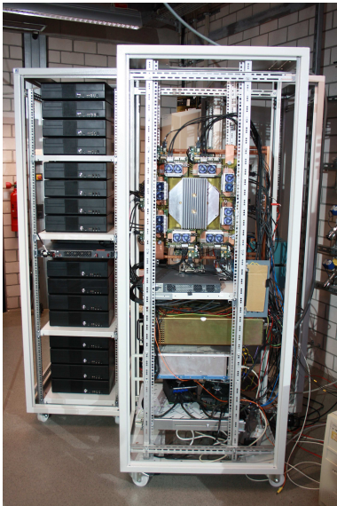
Figure 1.1.: (A) The BrainScaleS wafer-scale system in the lab. The left rack holds the cluster of control computers operating the neuromorphic system in the rack to the right. Here, the current variant with one wafer module is shown. Photo by S. Schrader. (B) Post-processed wafer. Photo by A. Grübl.
